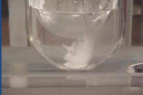
A new stirrer, known as Crescent-shape spindle, has been suggested. The stirrer (spindle) sits at the base the vessels and provides efficient stirring and mixing even at lower rotation speed of 25 rpm.
