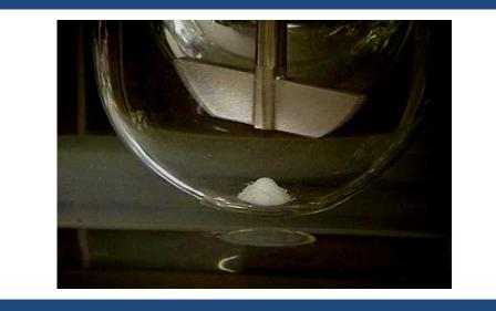
This picture is taken from a video clip of a dissolution test, demonstrating lack of stirring and mixing within dissolution vessels/apparatuses, essential for appropriate dissolution testing. Thus, it is not possible to obtain appropriate dissolution characteristics of a product.
