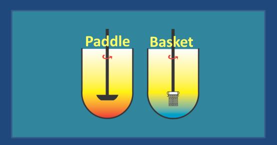
With rotation speed between 50 to 100 rpm – as per pharmacopeias e.g. USP
