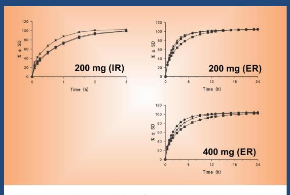
Dissolution characteristics of multi-vendor carbamazepine products using Crescent-shaped spindle (identical experimental conditions)
